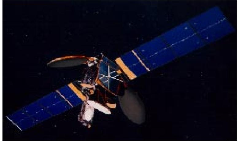
SS/L's 1300 platforms are designed to achieve long useful orbital life — in this case 10 years — through use of a bipropellant propulsion system and a momentum-bias system for excellent stationkeeping and orbital stability. Solar arrays and nickel-hydrogen batteries provide uninterrupted electrical power.
