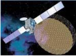
MBSAT-1 satellite SS/L successfully introduced the electric propulsion technology commercially on *MBSAT*, which was built for **MBCO (Mobile Broadcasting Corporation)** of Japan. Previously these thrusters were used on multiple Russian satellite missions and adapted for SS/L use after extensive ground tests for life, power electronics interfaces, and analysis of the plume impingement effects.
